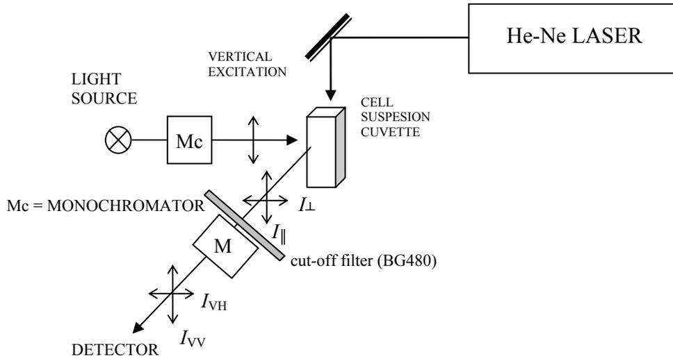
Fig. 1. – Experimental setup (optical scheme).
