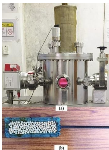
Fig. 1. Vacuum chamber (a), seeds holder (b).
